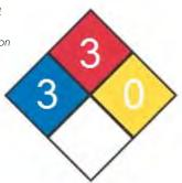
Figure 3. NFPA 704 Warning for Outdoor Ammonia Refrigeration Equipment
